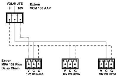
Figure 6. Regulating Multiple Amplifiers with a Single Volume Controller
